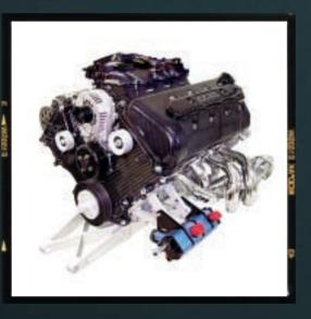
The CC8S' engine is fitted with carbonfibre cam and front covers, which reduce overall weight by about 12 kg compared to the same parts manufactured in aluminium. The highly efficient induction system is also made of carbonfibre; it is an advanced series of ducts and boxes, organically shaped to maximize the flow of air into the engine. The total weight of the Koenigsegg CC8S' engine is only 210 kg.
