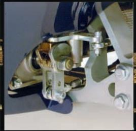
necessary due to the immense engine power. The final gear ratio is calculated to propel the car close to 400 km/h (250 mph) at 7.300 rpm. Koenigsegg also has engineered the unique anti-roll bars, essential to get superb handling qualities. They are operated by pushrods linked to each top wishbone. The function of the antiroll bar can easily be altered just by changing the cross-link to stiffer or softer ones.
