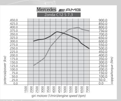
PAGANI ZONDA C12 S IS EQUIPPED WITH A MERCEDES-BENZ AMG ENGINE, 7.3 LITRES 12 CYLINDERS WITH 555 HP (408 KW) AND 750 NM TORQUE AT 4050 RPM. THIS ENGINE IS ENGINEERED AND BUILT WITH CRAFTMANSHIP DEDICATING ITSELF TO THE HIGHEST TECHNOLOGICAL STANDARDS.
