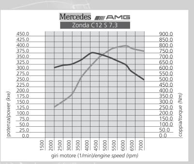
PAGANI ZONDA ROADSTER IS EQUIPPED WITH A MERCEDES-AMG ENGINE, 7.3 LITRES 12 CYLINDERS WITH 555 HP (408 KW) AND 750 NM TORQUE AT 4050 RPM. THIS ENGINE IS ENGINEERED AND BUILT WITH CRAFTMANSHIP DEDICATING ITSELF TO THE HIGHEST TECHNOLOGICAL STANDARDS.
